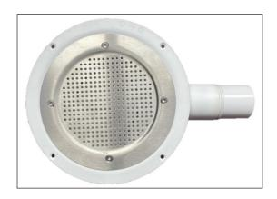
Purus' Anti-Ligature 59mm S-Series floor gully has an anti-ligature grate and is designed for use in health and care facilities with higher security requirements, as well as in prisons. It has a super-low profile of just 59mm and includes a NOOD no-odour water trap to ensure any foul smells are not omitted through the drain.
