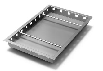
Sediment trap in acid-resistant stainless steel with a volume of 5.0 liters. Sand traps are used to collect smaller particles that are heavier than water, such as sand and gravel. These collect in the sediment trap at normal flows. The product is used, for example, when emptying scrubbers, car washes, dry cleaners.
