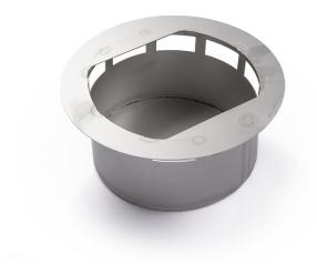
Sediment trap in acid-resistant stainless steel with a volume of 1.3 litres, designed to fit the Bigg and Heavy floor gullies, as well as the Kitchen Channels when used with an extension ring. Sediment traps are used to collect smaller particles which are heavier than water, such as sand and gravel. The particles collect in the trap, which can then be removed for emptying and cleaning.
