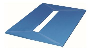
1600x900x22mm Linear Self-Supporting Wetroom Former Tray for the linear Purusline Living 800 and Purusline Living Plus 800. The former tray fits on top of concrete floors or wooden joists, and can be used with tiled or vinyl floor finishes. The outlet hole is positioned in the centre of the tray. Can be cut to size.
