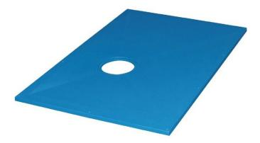
1500x800x22mm Self-Supporting Wetroom Former Tray for the 130mm diameter Mini Series floor gullies. The former tray fits on top of concrete floors or wooden joists, and can be used with tiled or vinyl floor finishes. The outlet hole is positioned off-centre to allow for avoiding existing joists. Can be cut to size.
